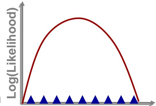
1 quadrature point Gaussian = Laplacian approximation
